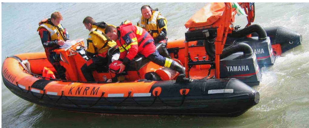
Figure 1 All AEDs became wet on the Atlantic type at normal sea conditions. Notice the limited space in which the AED had to be used.
